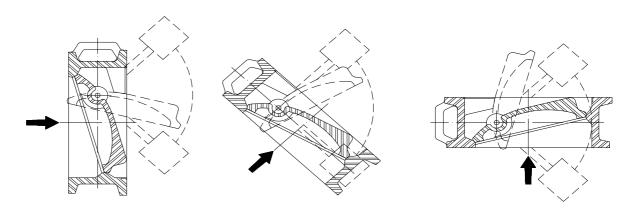
Valves installed in vertical lines must also be accurately centred. In all conventional applications, the valve must open upwards with respect to the direction of flow.
