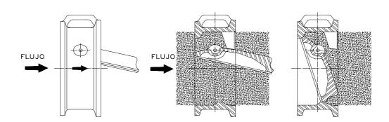
The valve should be mounted between two parallel flanges. It is essential that the valve is centred correctly between them to let the disc move freely. The valve is correctly centred when the distances between the external diameter of the flanges and the external diameter of the valve are the same through any diameter of the body valve.
