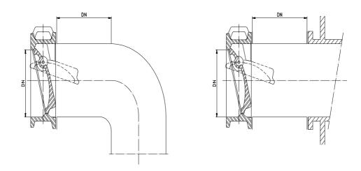
The position of the disc is also of vital to valve operation. Make sure that the axis of rotation of the disc is in a horizontal plane, regardless of the pipe position (see the following diagram).
