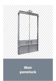
Three- or four-side sealing downward opening. Stainless steel frame and gate, EPDM seals and HMWPE guides, bidirectional and with various actuation solutions (manual, pneumatic, electric, etc.)
